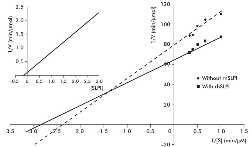
**Figure 2.** Lineweaver-Burk curve of the activity of porcine pancreatic elastase (PPE) without and with the obtained recombinant human secretory leukocyte protease inhibitor (rhSLPI). In the inset is depicted the secondary curve use for the calculation of the  $K_i$  value. V: enzyme reaction rate. S: substrate concentration, N-succinyl-L-alanyl-L-alanyl-L-prolyl-L-phenylalanyl-4-nitroanilide (NPN).
