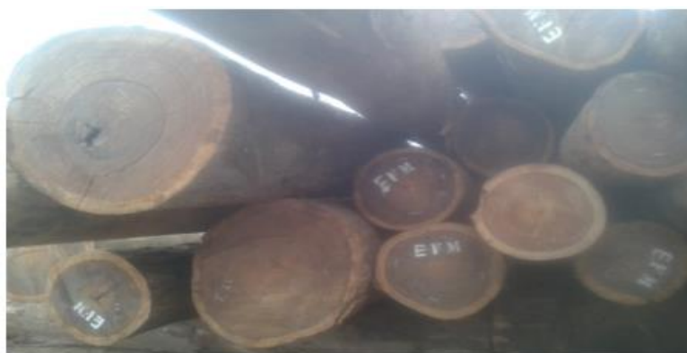
Figure 5 - Tiama logs with ovality
