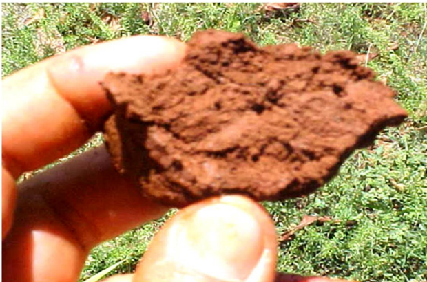
Photo 4. Angular block structure. Horizon Bt, Red Ferrallitic Leached soil. San José de las Lajas, Mayabeque, Cuba
