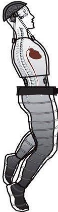
Fig. 2. Schematic of wearable LBNP-device. LBNP is generated from a portable vacuum powered by a battery. In addition to generating blood and fluid shifts towards the feet, mechanical forces are also generated by the vacuum. The negative-pressure trousers are attached to a vest and a cap to distribute the mechanical loads to the entire axial system. Use does not interfere with daily activity in space. Duration is limited by battery lifetime. (Petersen et al unpublished, with permission).
