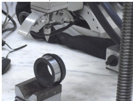
Fig. 2. Analyzer of stresses Stresstech, model X stress 3000
