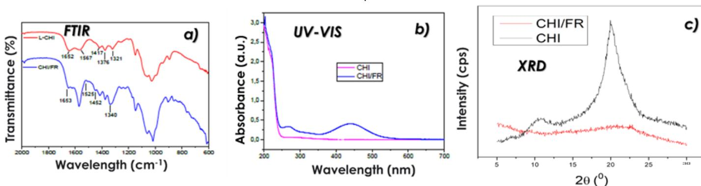
Fig. 1- a) FT-IR spectra, b) UV-VIS spectra and c) XRD patterns of CHI and the CHI/FR polymer dye
