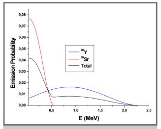
Figure 2. Energetic spectra of emission probabilities.
