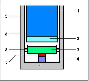
**Figure 1.** Experimental Arrangement Scheme: 1-Gamma Müvek ND-304 Scintillation Detector, 2-Detector's window (1 mg·cm²Al thin film + 1cm of air), 3-Sample, 4-Plastic base, 5-Lead shielding, 6-Air, 7-  $5 \mu \text{Ci}$   $^{90}\text{Sr}/^{90}\text{Y}$  Amersham source (E<sub>m</sub> = 2.28 MeV) and 8-Cylindrical plastic container (only when the sample is liquid).
