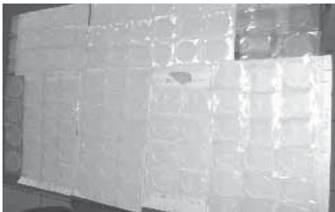
Figure 6. Hydrogel membranes dressing batch of PVP, Agar, PEG, and 90% of Water. Disc shape with size \varnothing = 100 mm, and \varnothing = 50 mm Irradiated with Electron Beam and Cobalt 60 irradiation facility at 25 kG, at the laboratory scale
