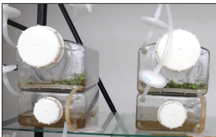
Figure 1. Temporary immersion systems SETIS™, used in the in vitro multiplication of mulberry sprouts, at 28 days of cultivation.
