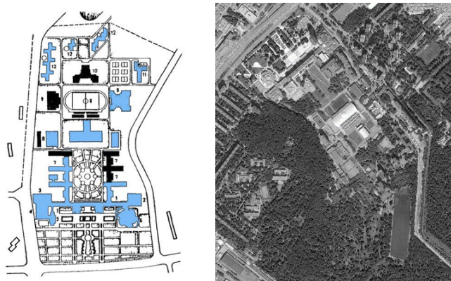
Figure 5. General plan and aerial photograph of the Moscow State University of Civil Engineering. Blue shows the implemented part of the plan (1 – junior year building; 2 – canteen; 3 – library; 4 – assembly hall; 5 – rectorate; 6 – classroom block; 7 – departments; 8 – service buildings; 9 – sports palace, swimming pool, arena, stadium; 10 – community center; 11 – preventorium; 12 – dormitories).
