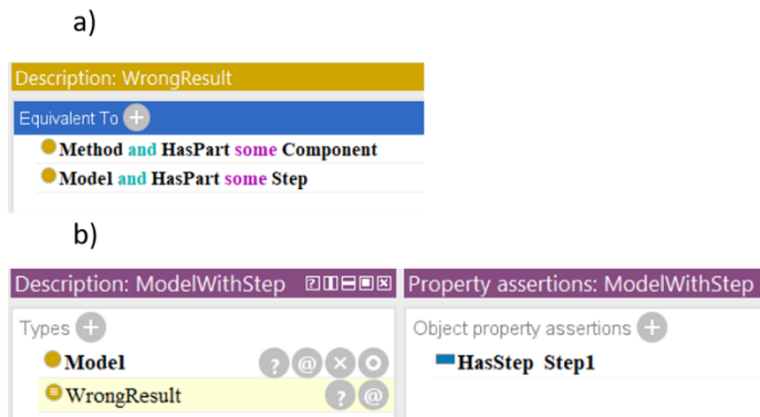
Fig. 6 - a) Necessary and sufficient conditions for the defined class and b) inference of a wrong result.
