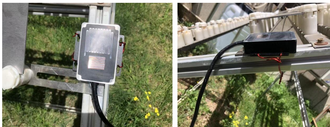
Fig. 3. ACMS to be installed in the coastal atmospheric corrosion station of Cuba.
