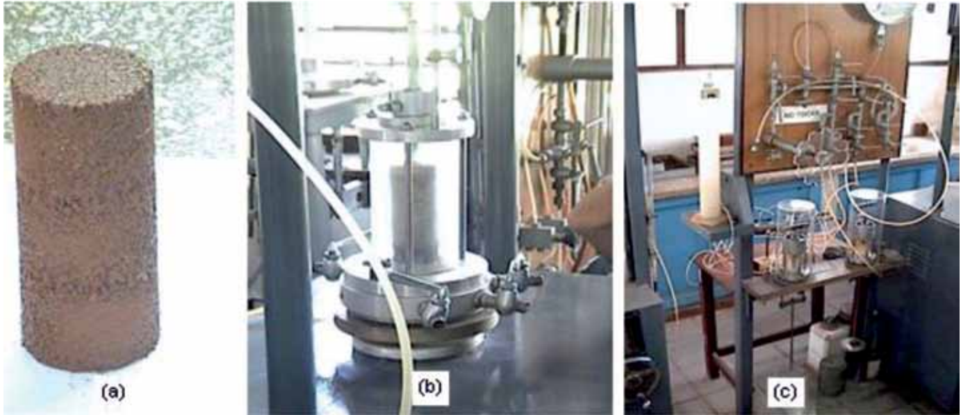
FIGURE 2. Triaxial compression test; cylindrical sample (a), water pressure recipient (b) and pressure system control (c).
