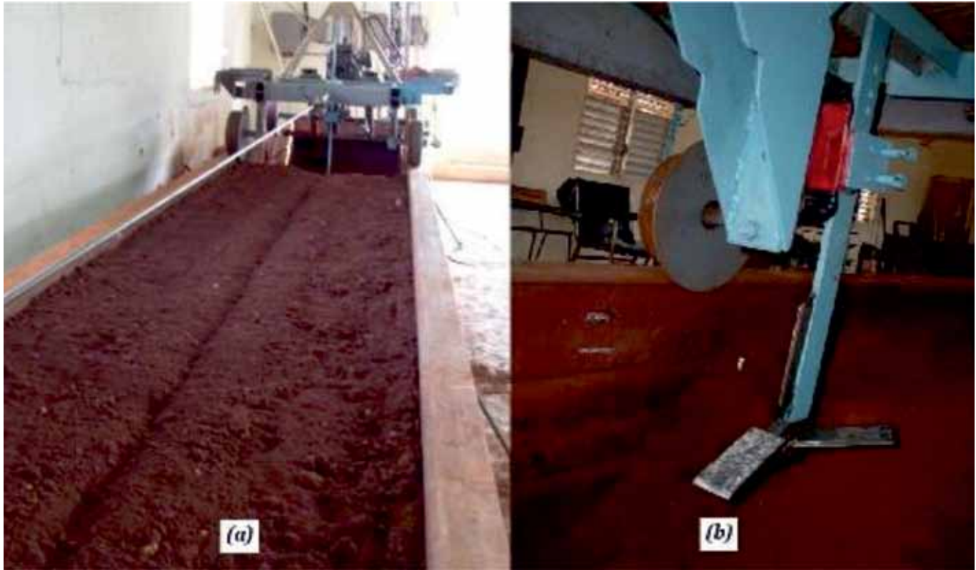
FIGURE 3. Soil-bin installation (a). Tool, transducer and trolley coupling (b).
