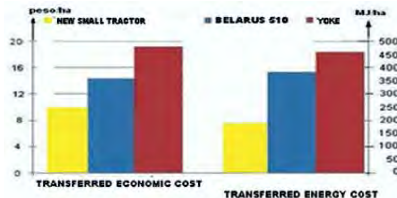
FIGURE 3. Behavior of Transferred Energy and Economic Costs of New Small Tractor With Cultivator “Camajuani”, BELARUS 510 Tractor Cultivator “Camajuani” and Animal Traction with Cultivator “Criollo”.
