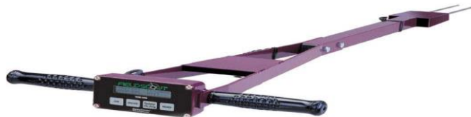
FIGURE 1. Probe TDR 300, model 6430FS, used in the determination of soil moisture content.
