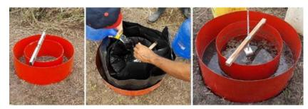
FIGURE 3. Placement of the Infiltration Rings for the determination of water infiltration rate at one of the observation points.
