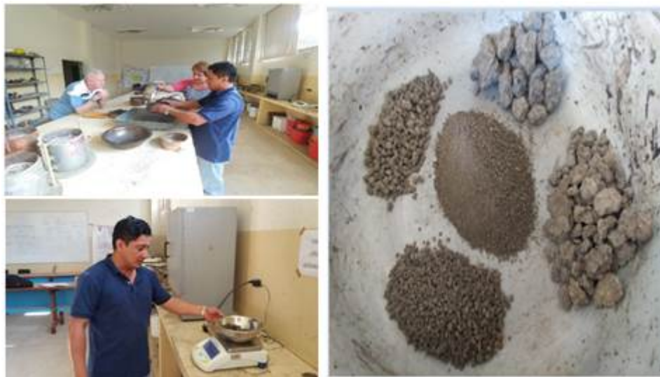
FIGURE 4. Granulometric analysis of soil by sizing.
