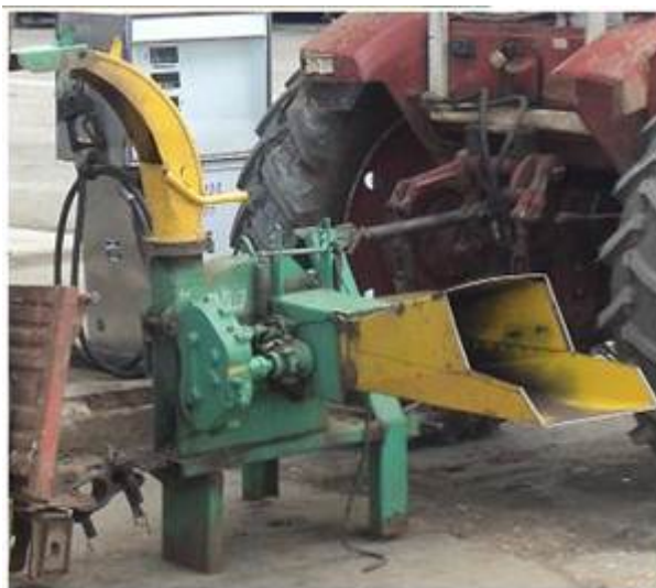
FIGURE 1. BELARUS 510-tractor and JF-50 forage chopper machine set.
