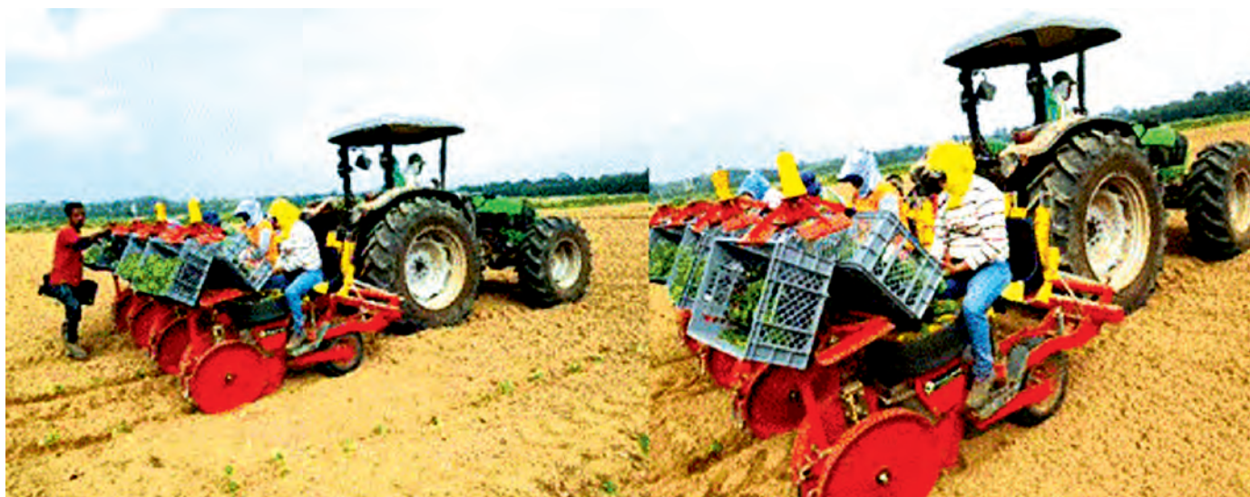
FIGURE 1. Deutz Fahr Agrofarm 420-T Ecoline Tractor and Checchi & Magli Transplanter Set FIGURA 1. Conjunto Tractor Deutz Fahr Agrofarm 420-T Ecoline y Trasplantadora Checchi Magli Unitrium. Source: Checchi & Magli (2012) and Ramirez & Shkiliova (2019).
