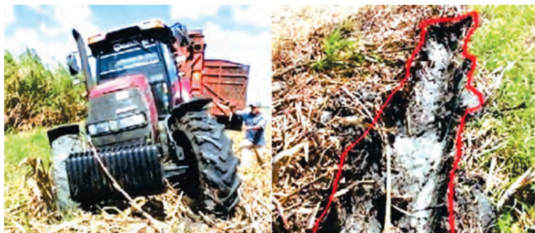
FIGURE 4. Intermediate transport in jam condition. FIGURA 4. Zona del atascamiento del transporte intermedio.
