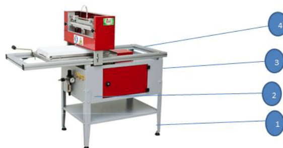
FIGURE 2. Tray seeding machine, 1- Support frame, 2- Movable tray support, 3- Seedling head, 4- Suction jar for seeds.
