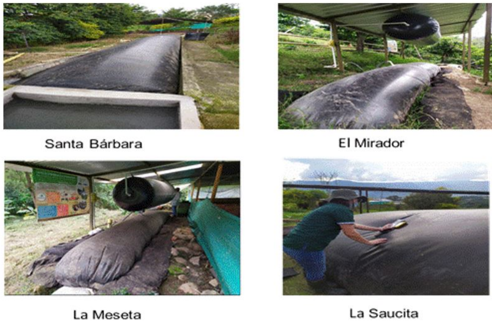
FIGURE 4. Membrane biodigesters evaluated in the experiment.
