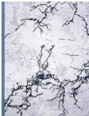
FIGURE 10. Under stress corrosion.
