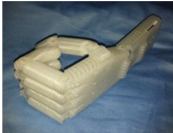
Fig. 2. Mechanical hand prosthesis materialized by additive manufacturing.
