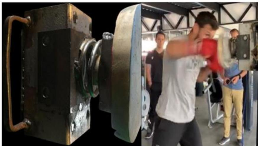
**Fig. 1.** - Metal structure for measurement of the maximum strength of the straight blow
