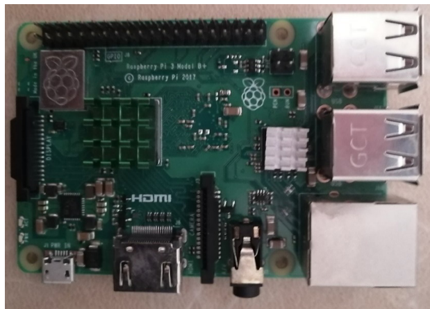
Figura 6. Raspberry Pi 3B+.
